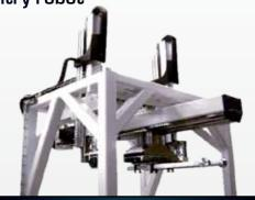
A robot integrating part stacking after removal from the IMM
