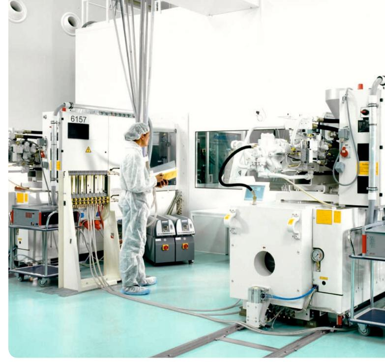
Intelligent production planning and the use of two-platen injection moulding machines makes it possible to comply with cleanroom standards up to Class 5 (DIN EN ISO 146444-1).
